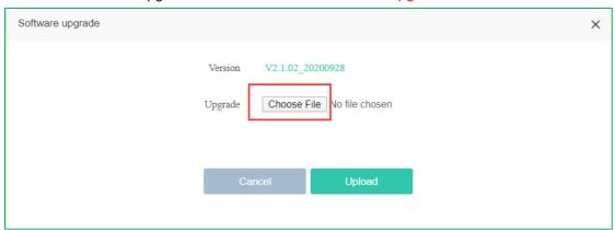
4. The way to select the file will pop up, select the file to be upgraded, click OK, the upgrade interface displays the name of the new software version, click OK to upload. (Note: The upgraded file format is bin format)
